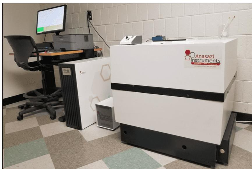
**Figure 1.** A Varian EM360 which has been upgraded through the Anasazi Instruments “Refresh Program” (<https://www.aiinmr.com/EM-360-NMR-Refresh-Program>). Image courtesy Anasazi Instruments
