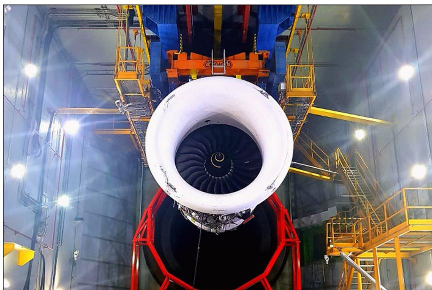
Researchers developed a technique called chemical species tomography that can capture carbon dioxide exhaust from a commercial airplane engine. To image such a large area, the researchers used a 7-m diameter optical mounting frame (red) located just 3 m from the exit nozzle of the engine. The testing facility is at the Instituto Nacional de Técnica Aeroespacial (INTA) in Madrid. Credit: Gordon Humphries, University of Strathclyde
