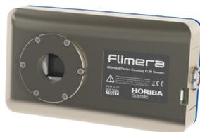
The FLIMera camera is a new concept in FLIM technology: a wide field imaging camera, rather than a confocal point scanning system, with the intrinsic benefit of acquiring FLIM dynamics at video rates, with time-correlated single photon counting measurements acquired independently in each pixel.
