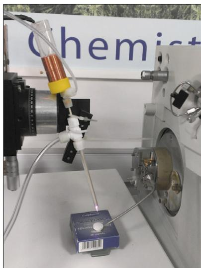
**Figure 2.** PADI set-up. The plasma flame interacts with a paracetamol tablet and resultant analyte ions are transported into the Waters ZQ single quadrupole mass spectrometer through a 1/8" stainless steel sniffer tube.
